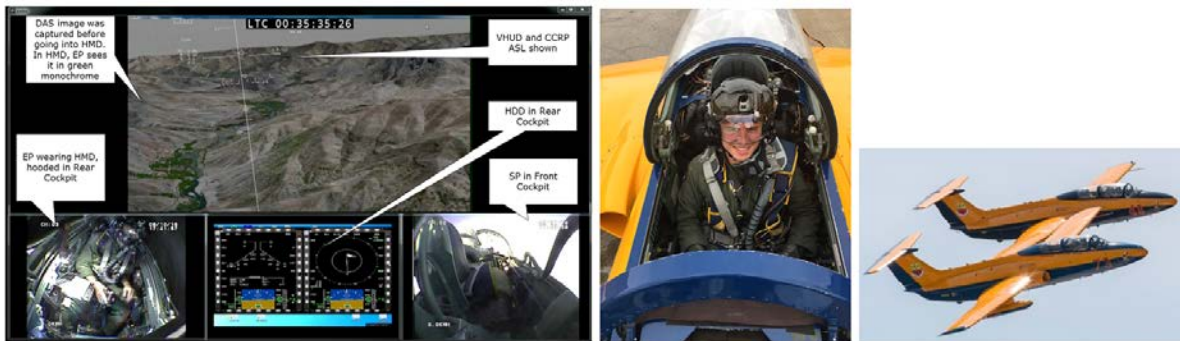
Figure 1. Fifth Generation Fighter HMD Integrated in OPL's L-29 Flight Testbed
