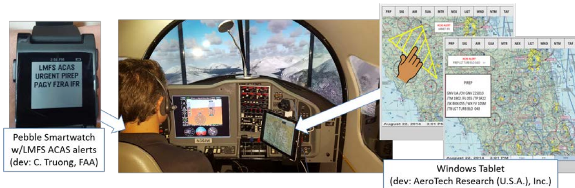
Figure 2. Flight training environment with weather alerts displayed as textboxes embedded in graphical display (right side, touch activated) and as text on a Pebble smartwatch worn by pilots on the left wrist.
