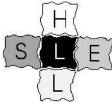
Figure 1. Diagram of SHELL components, with Liveware (human) in the center, surrounded by the Environment, and interacting with the Hardware and the Software and other Liveware (humans) (Hawkins, 1987).
