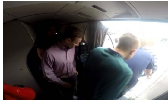
Figure 3. Camera mounted in the galley provided limited field of view in the cabin
