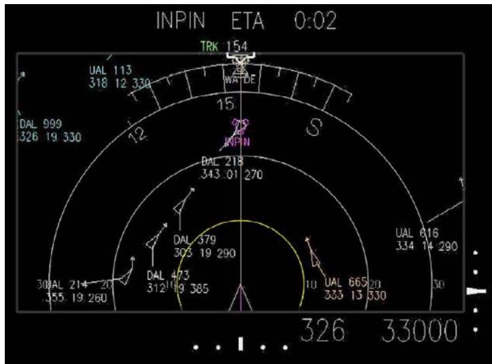
Figure 3a. A cockpit multifunction display showing range rings centered around the aircraft icon, b, upper) The gap function with and without a 20-nm range ring, b, lower) time-evolution of \rho , and areas of potential discernability, with and without 20-nm range ring.
