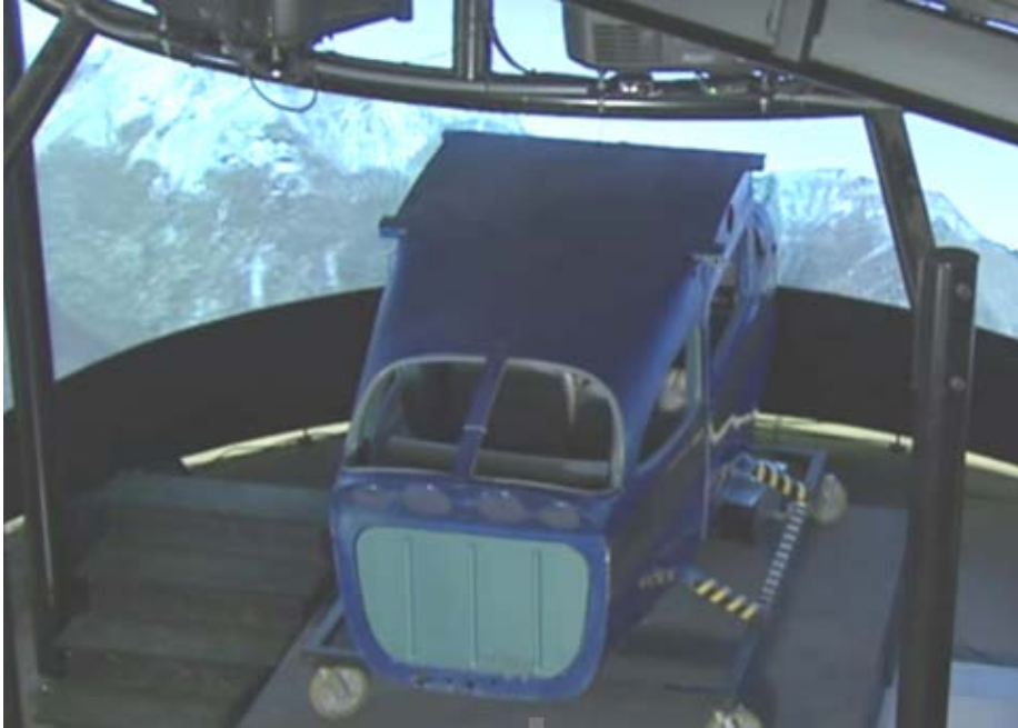
Figure 1. Cessna 172 simulator in situ with Broad-Angle Display System.
