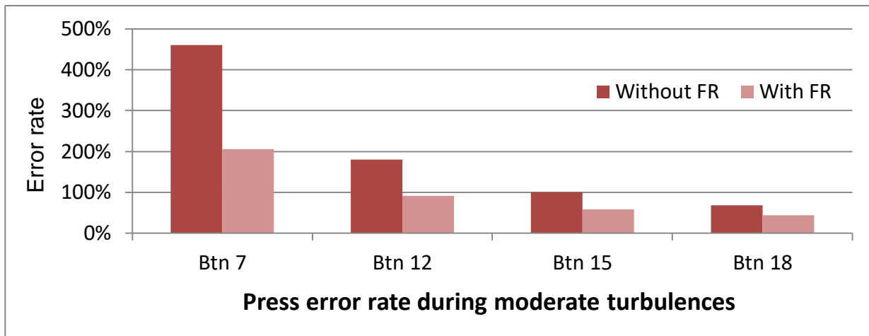
Figure 7: Error rate for various button sizes (in mm) with or without finger rest in moderate turbulence level.
