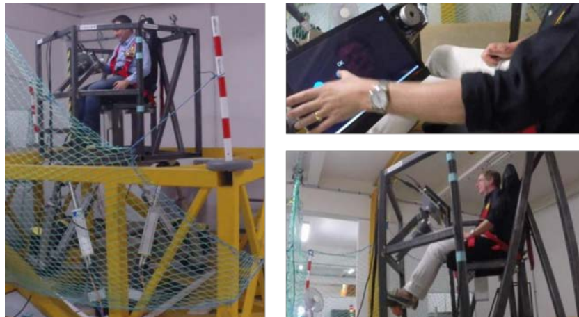
Figure 1: The Hexapod at ENSAM with the test bench on top
