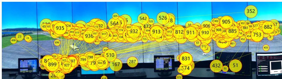
Figure 1. Visual scan path of an expert for a 10 minute period: Center of the circle is the eye fixation location, numbers indicate the time-ordered eye fixation sequences, and the yellow lines indicate the fast transitions among the eye fixations.
