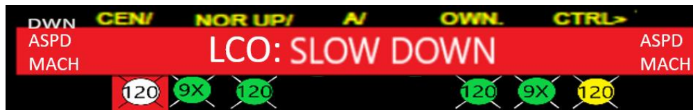
Figure 1: The left side shows the download envelope (DWN), and the right side shows the current envelope, both based on the current missile selected (shown in white). The LR banner appears when the participant was either: currently experiencing LCO, past their download limits, or out of bounds of their current flight envelope.
