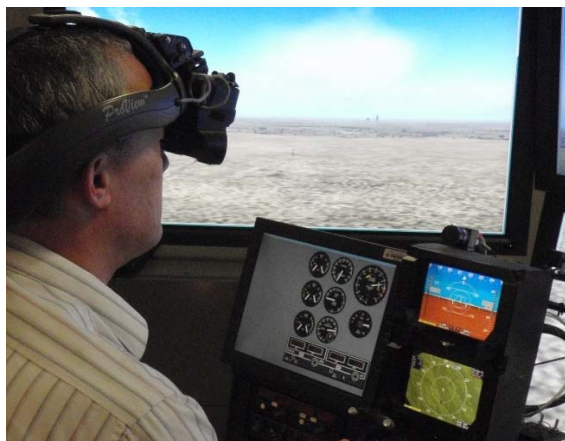
Figure 1. HMD and simulator cockpit with PFD/MFD, engine instrumentation, and out-the-window view.
