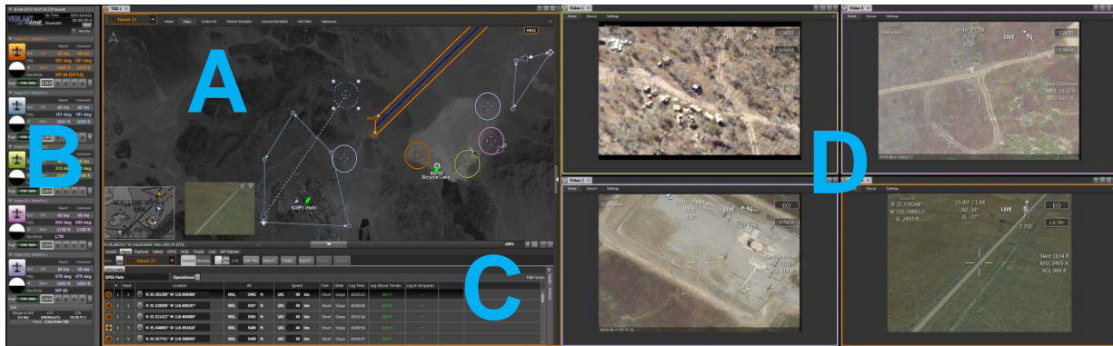
Figure 1. AFRL's Vigilant Spirit Control Station: An Example of a Multi-UAV Control Station. A) Tactical Situation Map, B) Vehicle Summary Information, C) Vehicle Management Panel, and D) Sensor Management.
