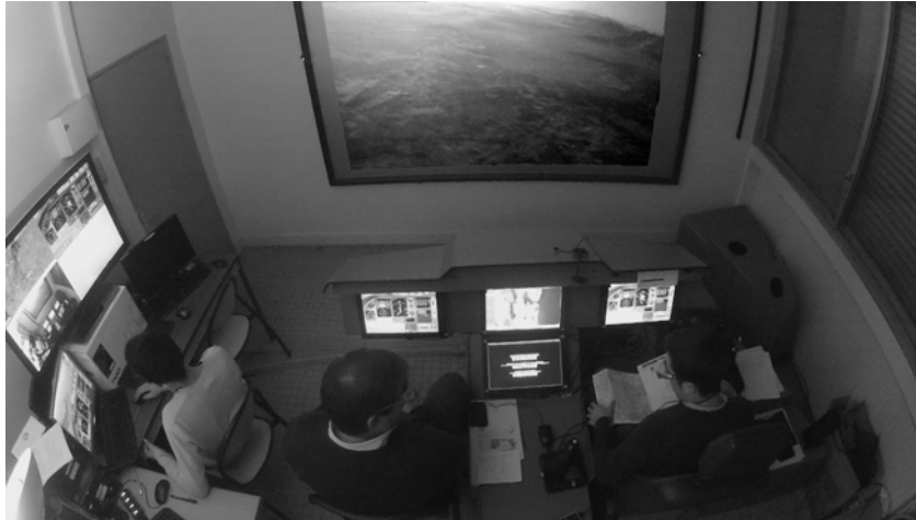
Figure 1: Overview of the simulator: the pilot flying (participant) was seating on the right, while a pilot non-flying was seating next to him on the left. The experimenter was monitoring from the left side of the room. Cockpit information was shown on the front panel while ASAP HMI was shown on the central upper screen and the 3D-SART on the central downer screen.
