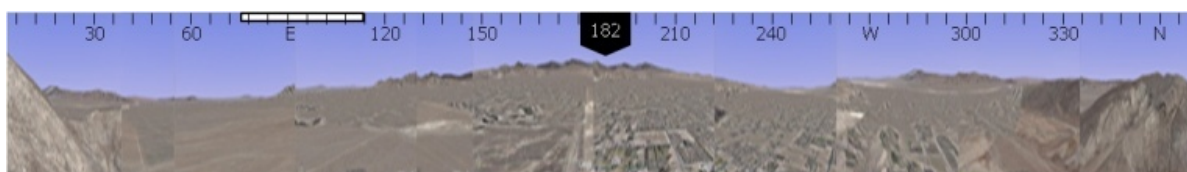
Figure 4. Panorama display. Compass tape is centered on vehicle direction of travel. White band represents camera field of view.
