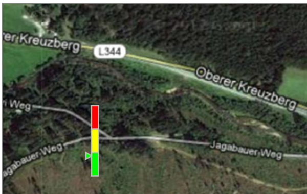
Figure 3. A model of the graphic interface of the early-warning system for landslide. The display shows multiple coding of the warning phase.
