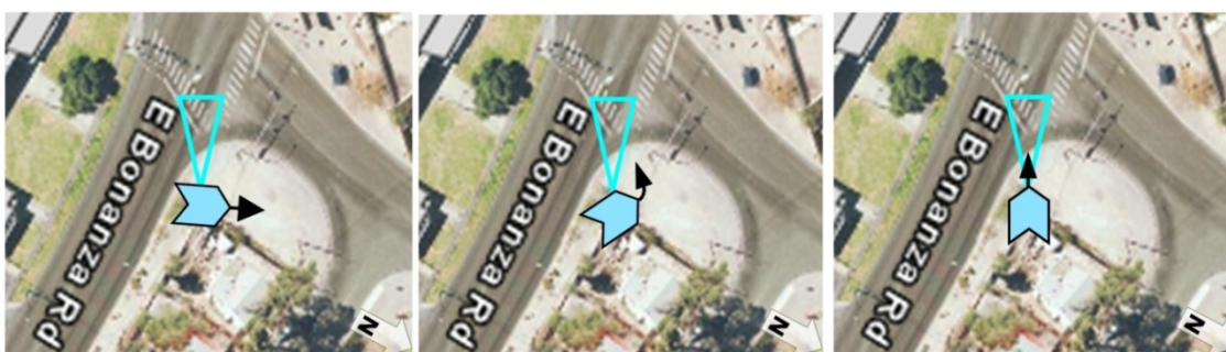
Figure 3. Camera-up map display as the operator turns to fly in the direction of the sensor (teal triangle).
