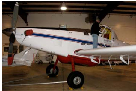
Figure 1. Air Tractor AT-802 SEAT aircraft, a turbo-prop designed for dropping chemicals from low altitudes.
