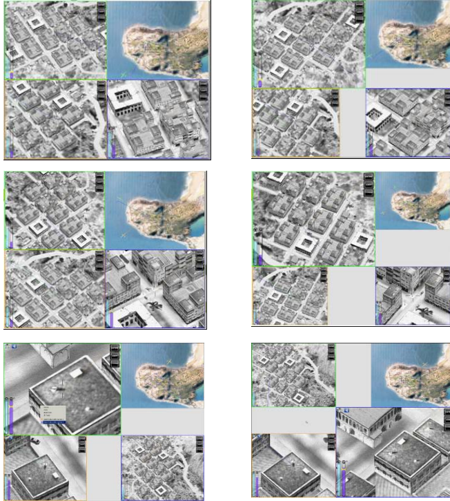
Figure 3. Example 1 (top): user defines a quality constraint on the upper left video (yellow line) (left). Window grows to maintain quality constraint (right). Example 2 (mid): bottom-right window has a quality constraint (left). Bottom-right window size decreases, system automatically zooms-in to maintain constraint (right). Example 3 (bottom): The operator desires to switch between the top-left payload (green) to the bottom-right payload (blue) (left). The video quality of the blue payload (zoom and window size) changes to maintain the quality definitions (right).
