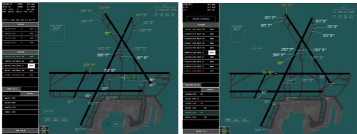
Figure 1. The TODDS ground (left) and local (right) control positions including FDEs, surface surveillance data, and weather information.
