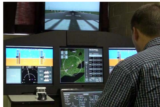
Figure 2. Prototype cockpit used in video prototyping evaluation.
