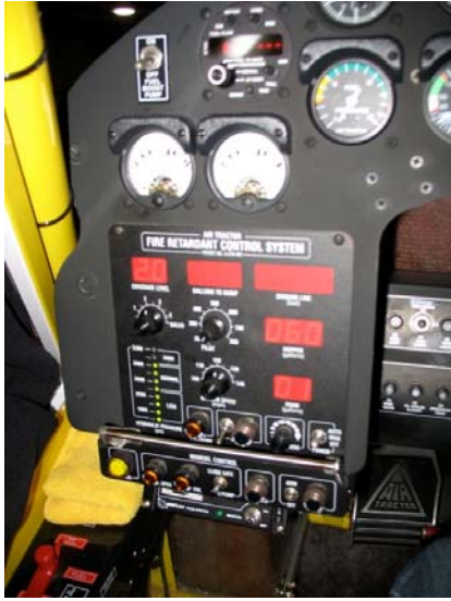
Figure 3. Typical AT-802 drop gate control panel (left) and radio control panel (right). While most SEAT pilots are already familiar with the drop gate controls due to their crop-dusting experiences, few have experience with the radio controls until they begin firefighting training.
