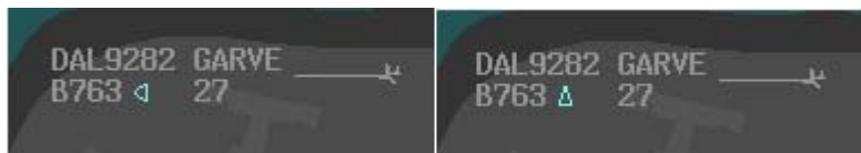
Figure 3. Data link indicator in data blocks for a pilot request (left), and a deferred request (right).
