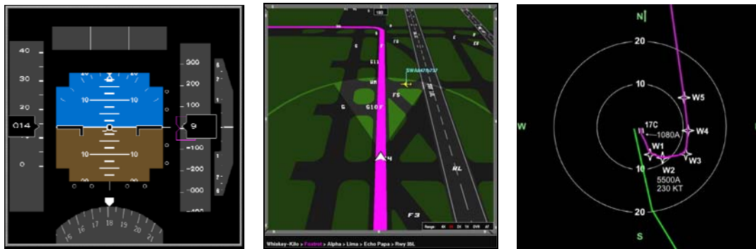
Figure 2. PFD (left), Taxi Navigation Display (middle), and Navigation Display (right).
