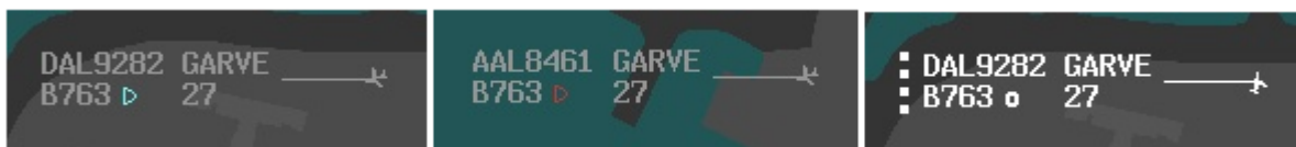
Figure 4. Data comm indicators in data blocks for a sent (left), failed (center), and accepted (right) D-Taxi clearance.
