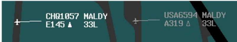
Figure 2. Data link capability indicators in the data blocks of owned (left) and unowned (right) aircraft.
