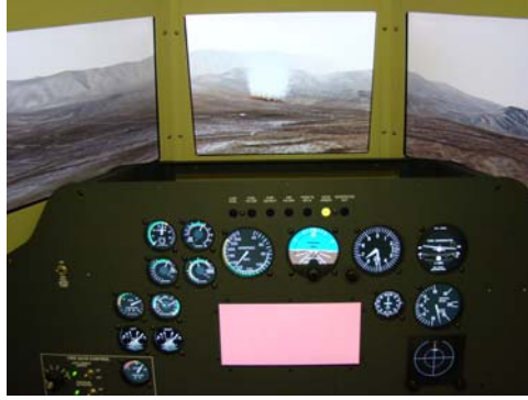
Figure 2. AT-802 prototypical cockpit simulator to be used for more rigorous initial and recurrent pilot training.
