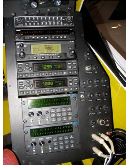
Figure 3. Typical AT-802 drop gate control panel (left) and radio control panel (right). While most SEAT pilots are already familiar with the drop gate controls due to their crop-dusting experiences, few have experience with the radio controls until they begin firefighting training.
