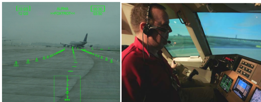
Figure 5. Surface HUD / HWD Displays
