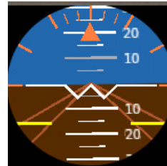
Figure 6. Throttle guidance indicator prompting an increase in energy state.
