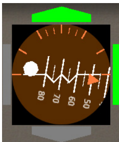
Figure 4. Roll and pitch indicators commanding a right bank and a pull up.
