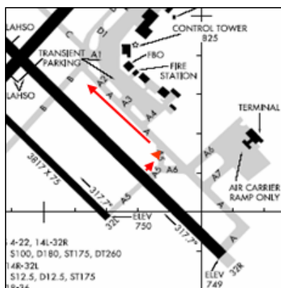
Figure 1. The nominal (experientially & spatially intuitive) taxi route used during all but the final trial of the second day.
