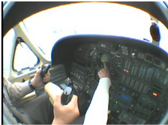
Figure 1. In this view from the HatCam, the instructor shows the student his pitch target for rotation during the takeoff.
