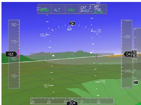
Figure 2 SVS showing a perspective view on the surrounding terrain.
