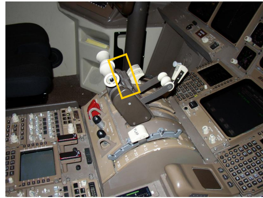
Figure 1. Boeing 777 throttle quadrant with TOGA switch highlighted.
