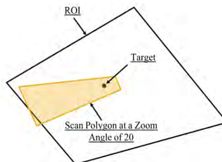
Figure 2. Target was classified as found if there existed a scan polygon (yellow) that happened below a zoom angle of 20 and the target was within the polygon.
