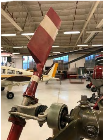
Figure 2. Schweizer 269A tail rotor used as a guide for the construction of the CATIA model
